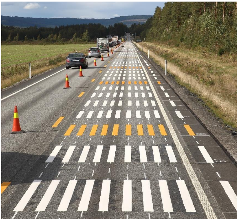
Figure 1. Materials applied at the Icelandic-Norwegian-Swedish test site. (Photo: Trond Cato Johansen, Ramboll).
